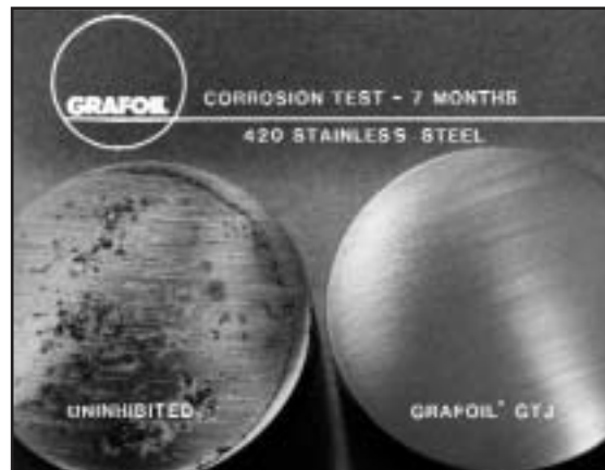
Figure 12 Photograph Showing How Inhibited GRAFOIL Grade GTJ Reduces Pitting Corrosion
